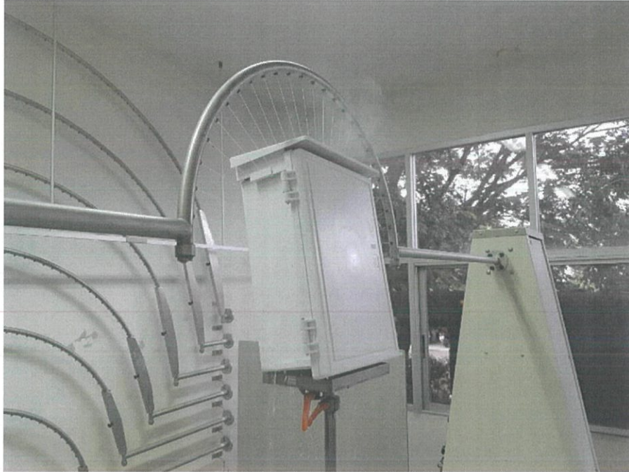
Photo No.5 : IPX4 Water test
