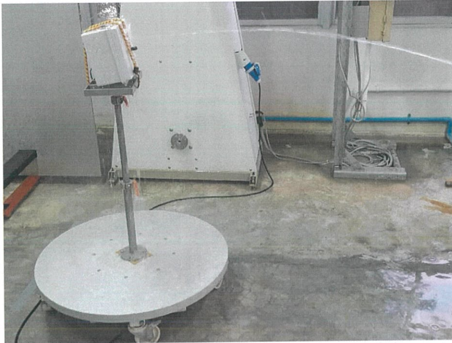
Photo No.5 : IPX5 Water test
