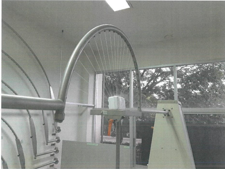
Photo No.5 : IPX4 Water test
