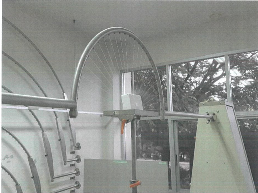
Photo No.5 : IPX4 Water test
